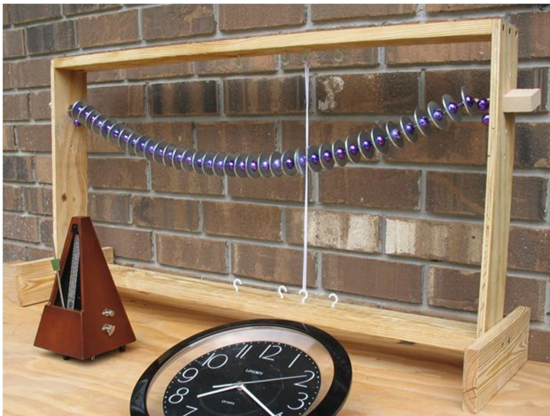
Figure 9: Set-up used to determine the frequency of oscillations of the horizontal string for different positions of the vertical barrier.
