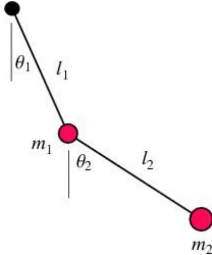
A double pendulum consists of one pendulum attached to another. Consider a double bob pendulum with masses  $m_1$  and  $m_2$  attached by rigid massless wires of lengths  $l_1$  and  $l_2$ . Further, let the angles the two wires make with the vertical be denoted  $\theta_1$  and  $\theta_2$ , as illustrated above. Finally, let gravity be given by  $g$ . Then the positions of the bobs are given by
